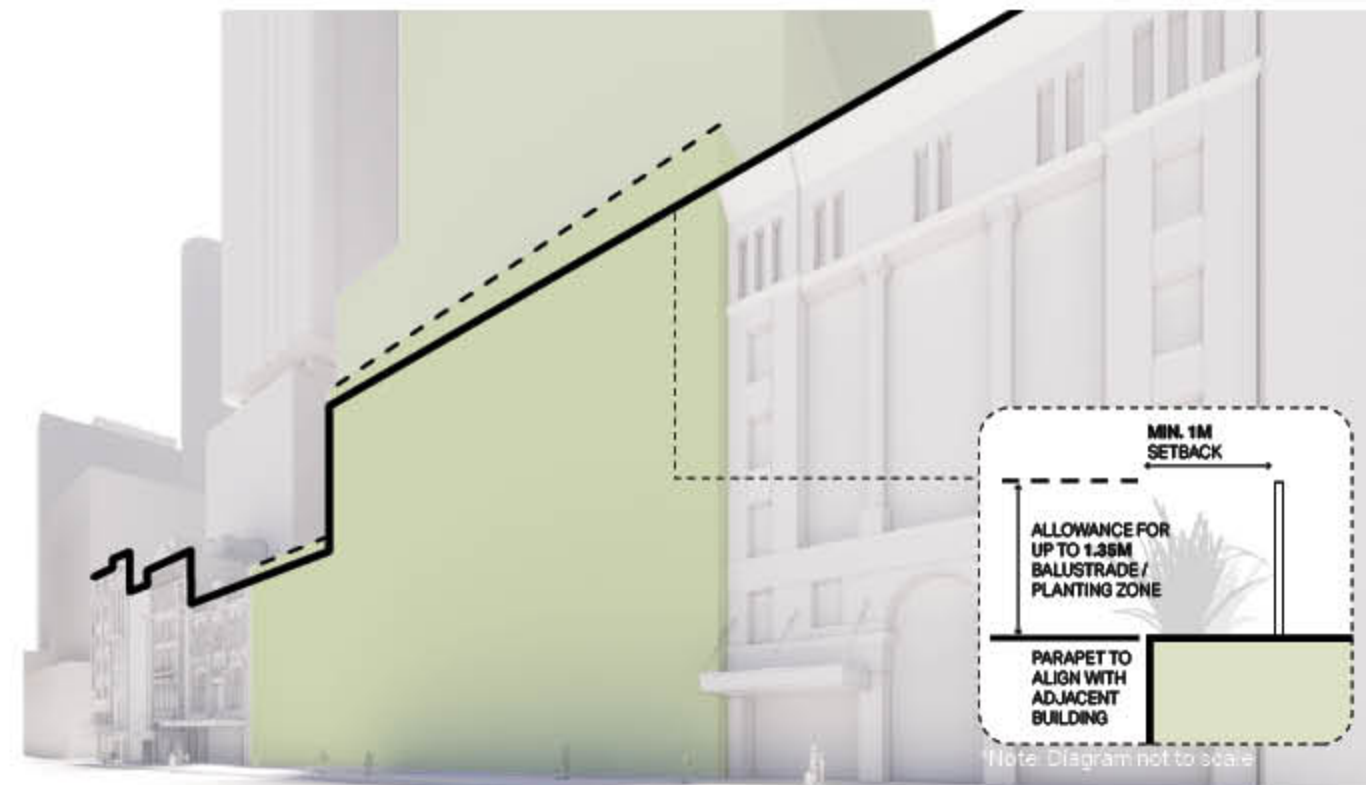
Proposed Envelope Close-up - Pitt Street, looking north.
